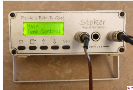
Figure 1. Rock's BBQ Stoker device with attached thermometers.
